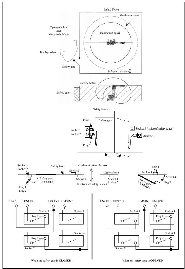
Fig.3.7 SAFETY FENCE and SAFETY GATE example
